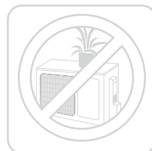
Make sure nothing is blocking all air inlets and outlets
