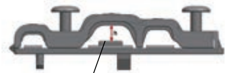
If the cable is not secured well, use the buckle to prop it up, so it can be clamped tightly.
